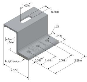
3 holes are provided for versatility. Some installations require only 2 fasteners. See the load table on the S-5I website and the installation instructions for more details.
